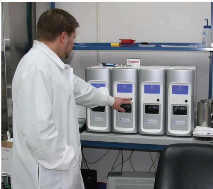
Keith Rando, medical lab technician at our Operations Center, is displaying the Verigene® System from Nanosphere, which uses microarray technology for characterizing isolates in positive blood cultures.
